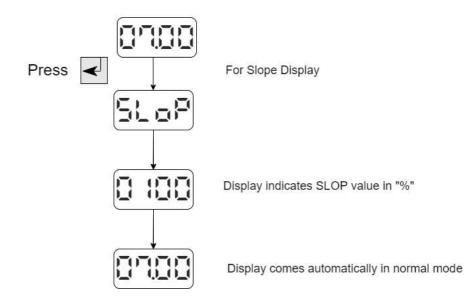
Slope indicates health of pH Sensor. Generally slope between **70 and 115%** is acceptable. If slope is below 70% or above 115%, you need to change the pH Sensor.
